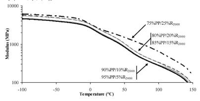
Figure 8. Storage modulus versus temperature, as a function of  $R_{2000}$  content.
