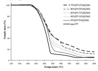
Figure 2. Thermogravimetric curves obtained on neat PP and  $PP/R_{2000}$  blends under oxidizing atmosphere.
