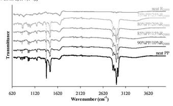
Figure 5. Infrared spectra of  $PP/R_{2000}$  blends. Curves have been shifted for clarity.
