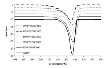
Figure 3. Derivative thermogravimetric curves obtained on blends  $PP/R_{2000}$  and neat PP under  $N_2$  atmosphere.
