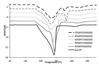
Figure 4. Derivative thermogravimetric curves obtained on blends  $PP/R_{2000}$  and neat PP under  $O_2$  atmosphere.
