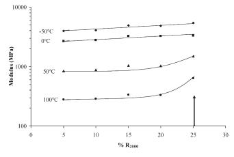
Figure 9. Storage modulus versus R2000 content, as a function of temperature (-50 °C, 50 °C and 100 °C).
